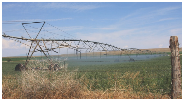
Figure 1. A typical and basic Center Pivot Sprinkler. Photo by author.
